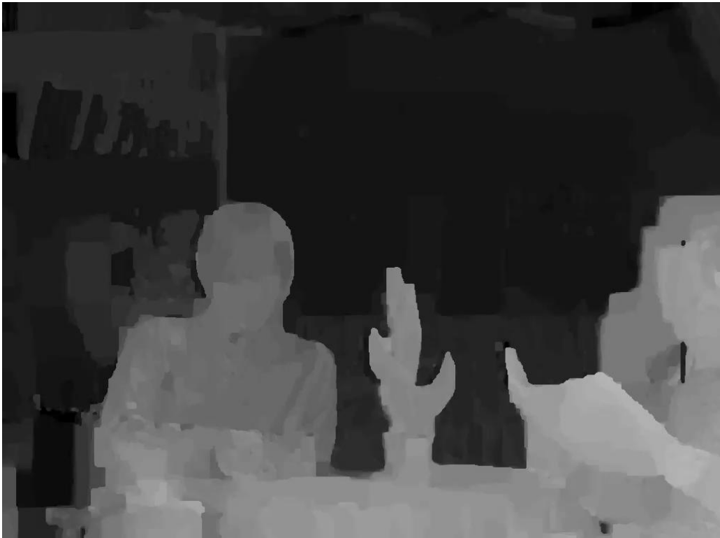
(b) The 10 th frame of the decoded depth map Newspaper view 2 resulted from Full Search using JM18.1
