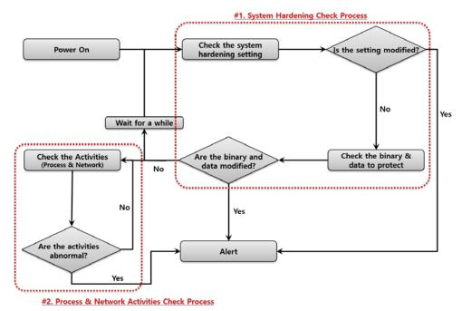
Fig. 6. Overall operation process
