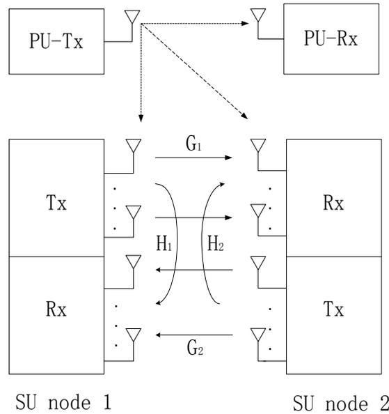
Fig. 1. FD-SSU-MIMO cognitive radio network model
