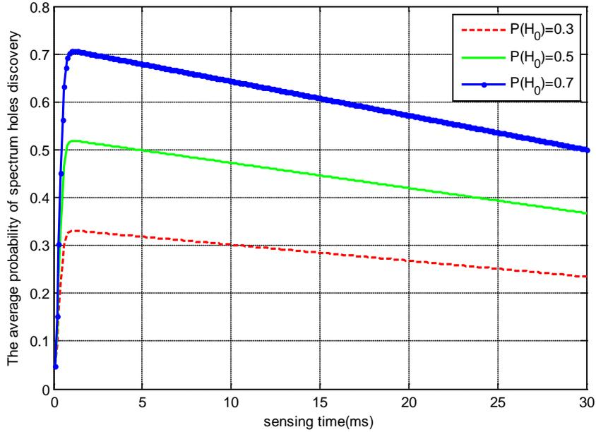
Fig. 3.  $F(\tau)$  vs. sensing time  $\tau$  with  $T=100$ ms
