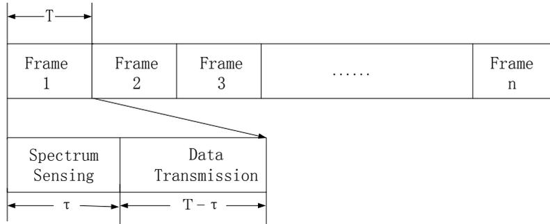
**Fig. 2.** Frame structure design for the CR network
