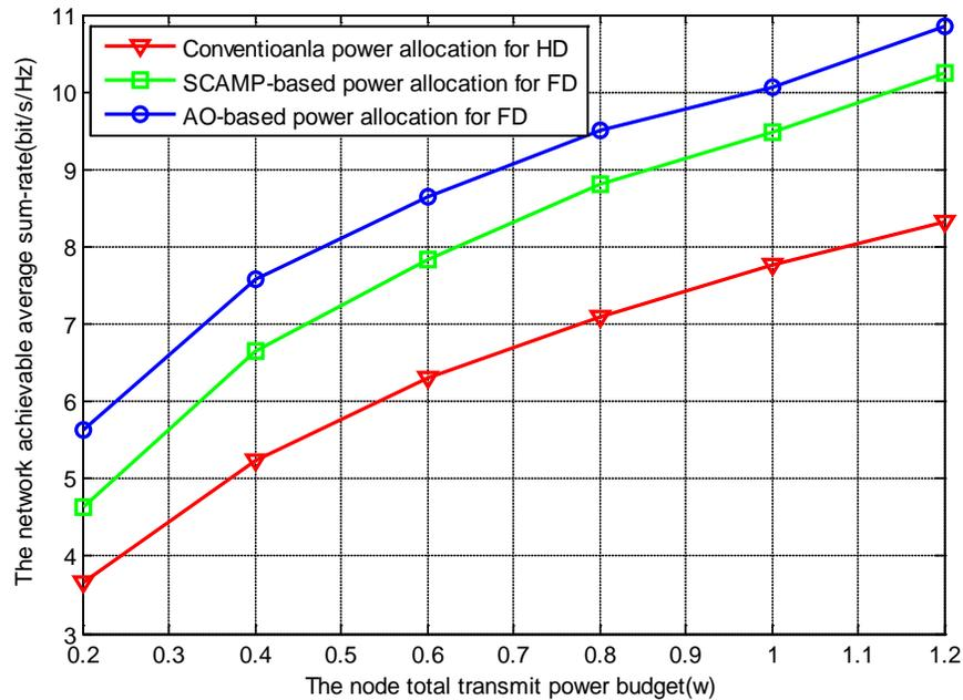
**Fig. 5.**  $R_{OSA}$  vs.  $P_{max}$  with  $N_t = M_r = 4$ ,  $SIR = -10\text{dB}$ ,  $SNR = 10\text{dB}$ ,  $\sigma_e^2 = 1$
