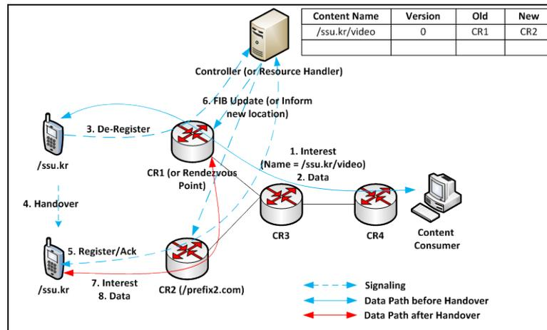
Fig. 5. Control Data plane separation-based approach operation
