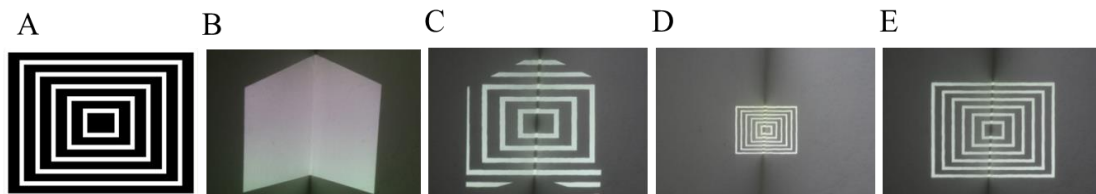
Fig. 2. Different compensation results according to setting of the compensation area: (A) Original input image to be projected to a bent surface; (B) Projection range of the project indicated by the gray regions; (C) A compensated image when the compensation area is set outside the projection range; (D) A compensated image when the compensation area is set very small inside the projection range; (E) A compensated image of the proposed method.
